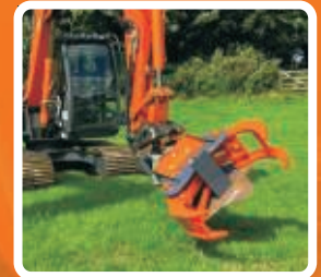
The shear comes with a custom-made Hydraulic cylinder which offers the force behind every cut.
